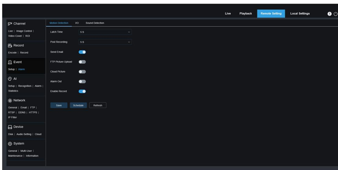
**Latch Time:** Set the external alarm triggering time when motion is detected.
