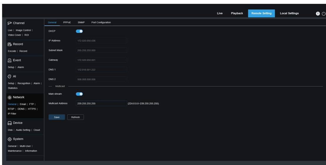
If connecting to a router that allows the use of DHCP, check the DHCP box. The router will automatically assign all network parameters to the camera unless you manually set the following parameters for the network:
