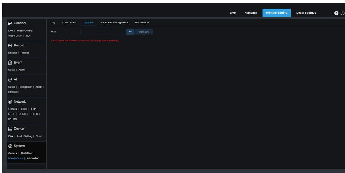
1. Put the firmware file (.sw file) on the computer hard disk.
