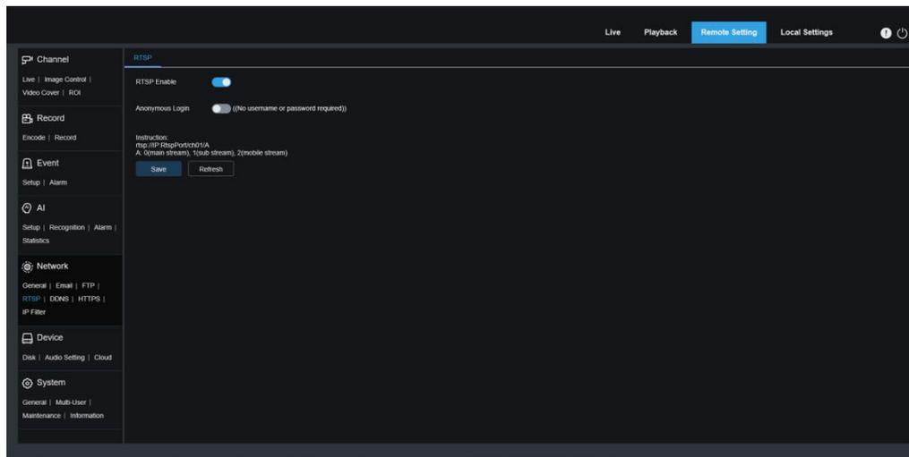
**RTSP Enable:** Turn on/off .This protocol can be used only after it is on.
