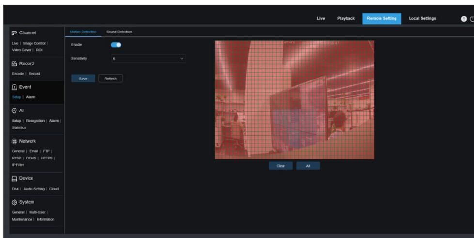
Drag the left mouse button to delimit the detection area in the right window. Only movement in the area will trigger an alarm.
