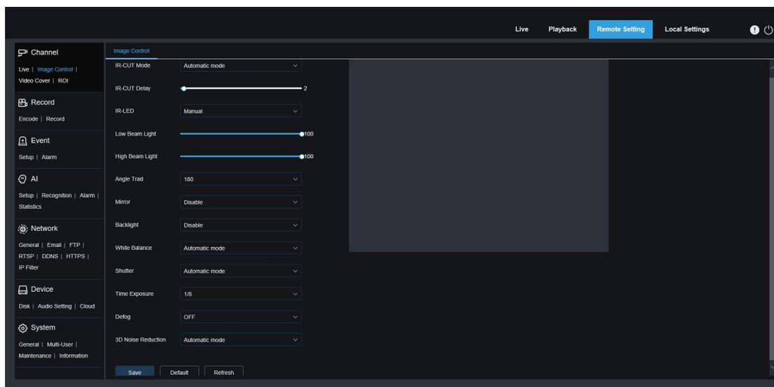
**IR-CUT Mode:** Set the day/night switching mode of the camera, a total of 5 modes.
