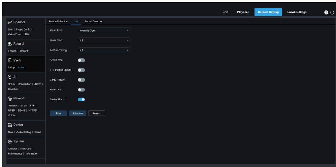
**Alarm Type:** Three types are optional: Normally open, Normally close and Off. Select a type that matches your sensor type, or select "Off" to turn off the sensor trigger function.
