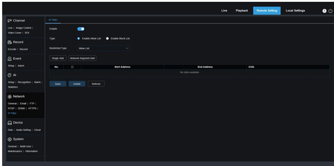
**Enable:** Enable or disable filter function. After enabling, allow list and block list are optional.
