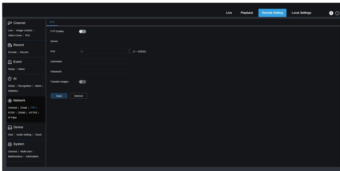
**FTP Enable:** Click to enable FTP function.
