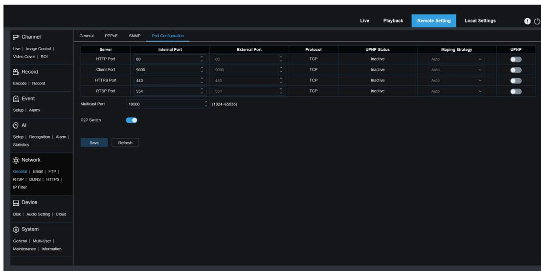
**Web Port:** This is the port you use to log in to the IPC remotely (for example, using a web client). If other application is already using port 80, please change it.
