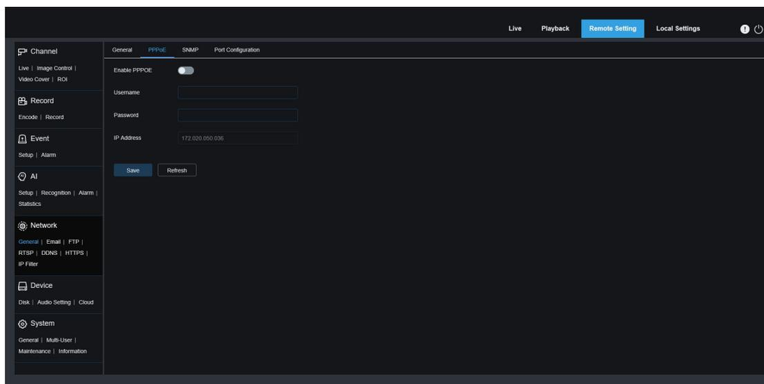
This is an advanced protocol that allows IPC to connect more directly to the network through a DSL modem.
