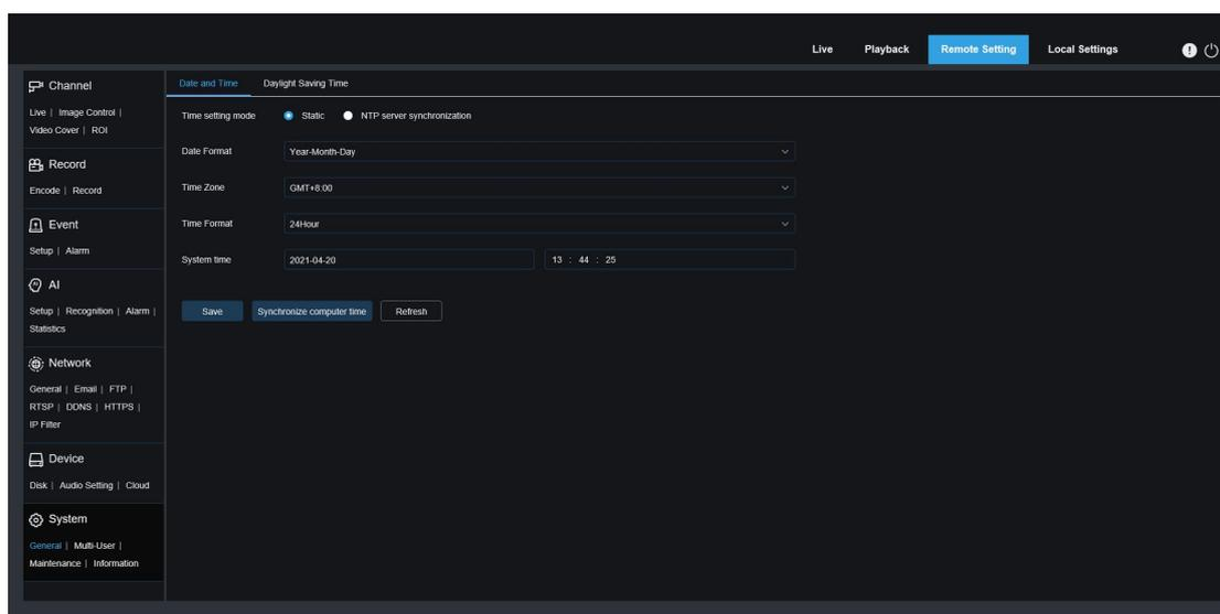
**Time setting mode:** Time mode, there are static and NTP synchronization optional. Static time needs to be set by yourself, while NTP synchronization will perform time calibration via network.
