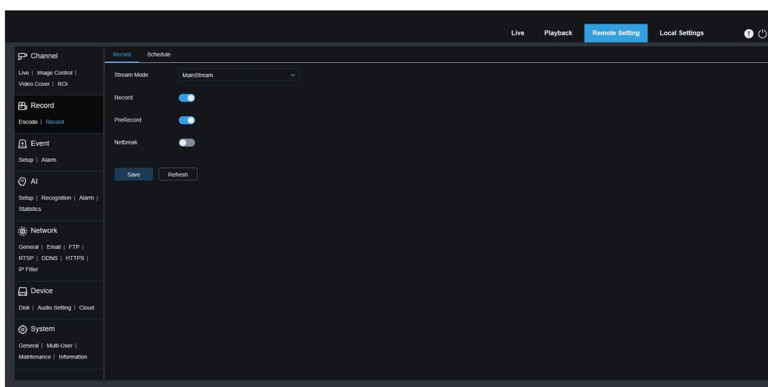
**Stream Mode:** The video stream to be saved in the SD card in recording mode. The default is the main stream.
